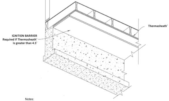
1. Refer to local building codes for requirements on proper ventilation and bracing.
