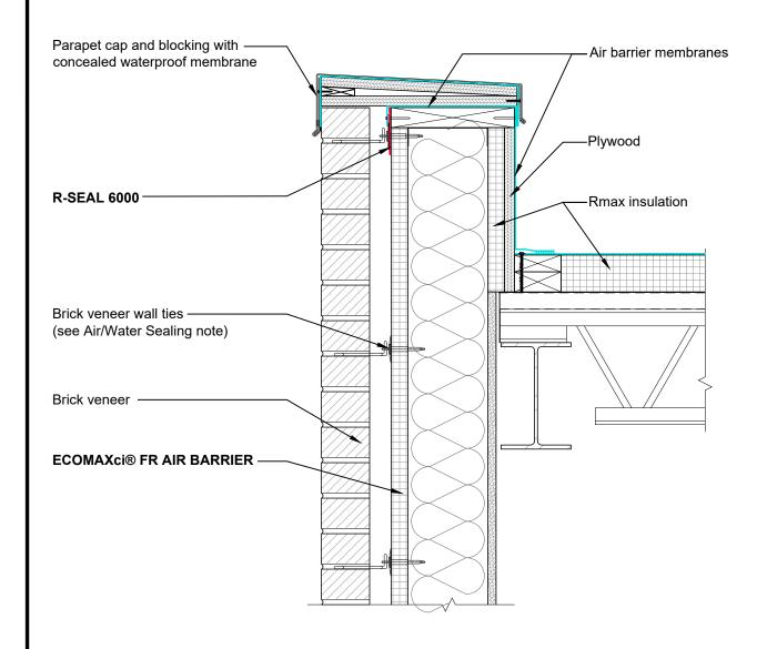
These details are graphical representation, not necessarily to scale and various features may be exaggerated. These details are intended to supplement the ECOMAXci® Wall Solution Installation Instructions located at www.Rmax.com, which should be consulted for additional guidance and installation requirements. Where discrepancies occur, the installation instructions supersede these details.
