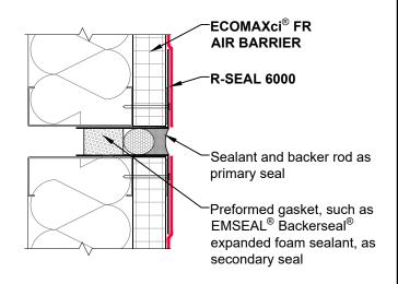
These details are graphical representation, not necessarily to scale and various features may be exaggerated. These details are intended to supplement the ECOMAXci® Wall Solution Installation Instructions located at <a href="www.Rmax.com">www.Rmax.com</a>, which should be consulted for additional guidance and installation requirements. Where discrepancies occur, the installation instructions supersede these details.
