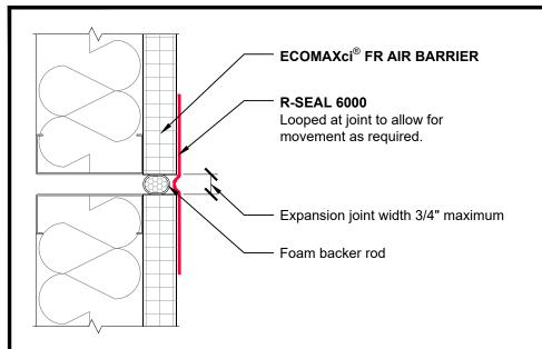
Note: Vertical expansion joint shown. Refer to deflection joint details for horizontal joint conditions.
