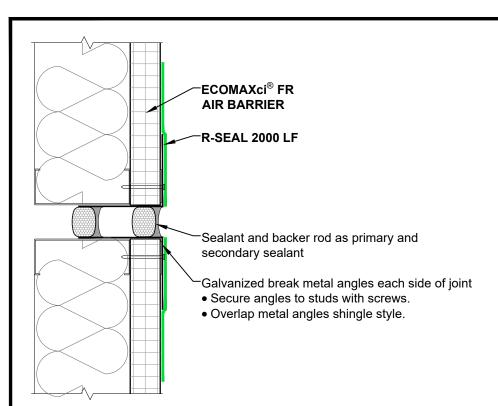
Note: Vertical expansion joint shown. Refer to deflection joint details for horizontal joint conditions.
