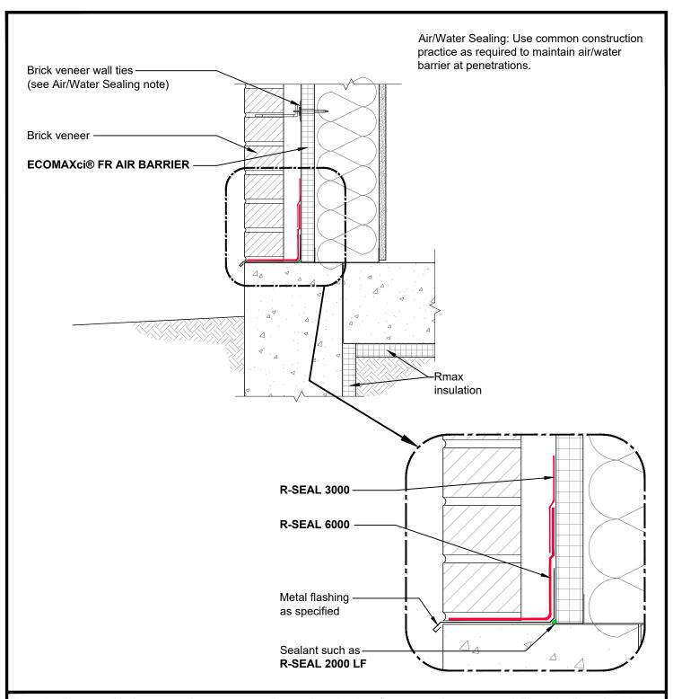
These details are graphical representation, not necessarily to scale and various features may be exaggerated. These details are intended to supplement the ECOMAXci® Wall Solution Installation Instructions located at <a href="www.Rmax.com">www.Rmax.com</a>, which should be consulted for additional guidance and installation requirements. Where discrepancies occur, the installation instructions supersede these details.
