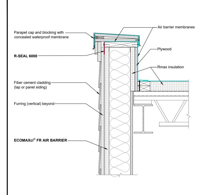
These details are graphical representation, not necessarily to scale and various features may be exaggerated. These details are intended to supplement the ECOMAXci® Wall Solution Installation Instructions located at www.Rmax.com, which should be consulted for additional quidance and installation requirements. Where discrepancies occur, the installation instructions supersede these details.
