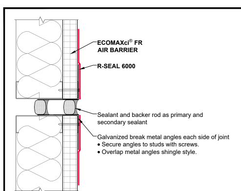
Note: Vertical expansion joint shown. Refer to deflection joint details for horizontal joint conditions.
