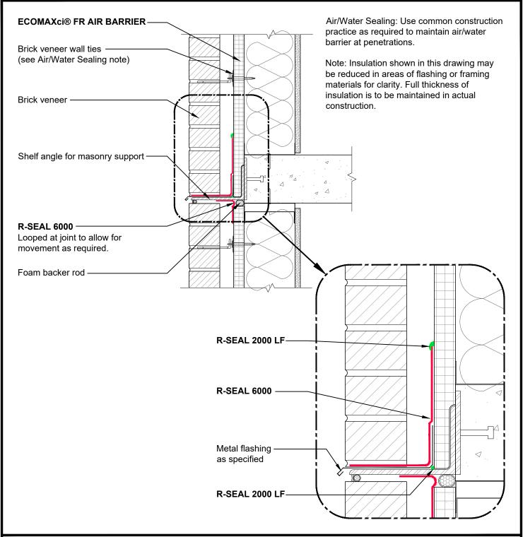
These details are graphical representation, not necessarily to scale and various features may be exaggerated. These details are intended to supplement the ECOMAXci<sup>®</sup> Wall Solution Installation Instructions located at <a href="https://www.Rmax.com">www.Rmax.com</a>, which should be consulted for additional guidance and installation requirements. Where discrepancies occur, the installation instructions supersede these details.
