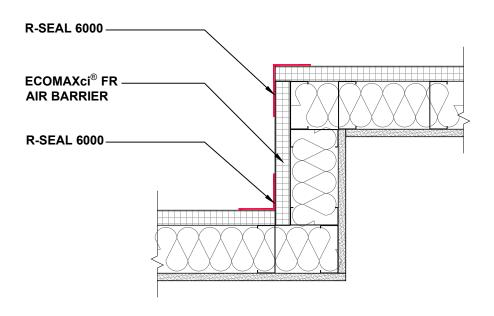
Provide sealant incorner to fill void prior to installing flashing tape.
